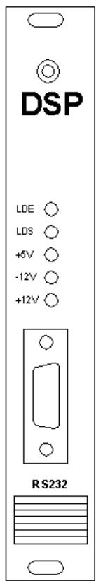
The DSP's status indicator are divided into two parts. One part is power supply including  $\pm 12V$  and  $+5V$  for DSP. The other includes two LEDs shown below. LDE is red. LDS is orange. There are three ways of blinking. Each blinking means a different motion mode or monitor mode. About motion modes, please refer to command 'FX' of "LMDX Command and parameter manual.pdf "
