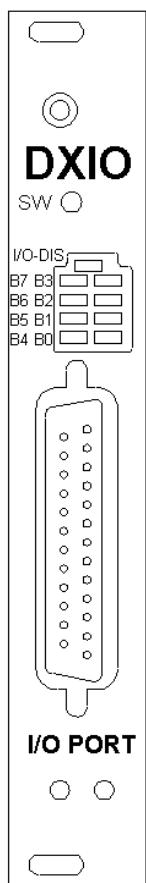
LEDs of DXIO card show LMDX input/output statuses. SW is a switch. It switches between input/output statuses. If I/O-DIS light, the status is input. Otherwise, it is output. The status is output when driver power on. So they can help users to see current status. Each LED is described below.
